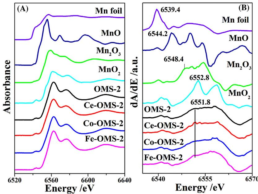
**Fig. 7.** (A) XANES and (B) first-order derivatives of XANES of MnK-edge in series of MnO<sub>x</sub> catalysts and Mn-containing reference samples.
