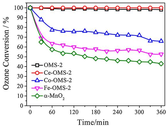
**Fig. 1.** The conversion of ozone on the OMS-2, M-OMS-2 and  $\alpha$ -MnO<sub>2</sub> catalysts at RH = 45%.
