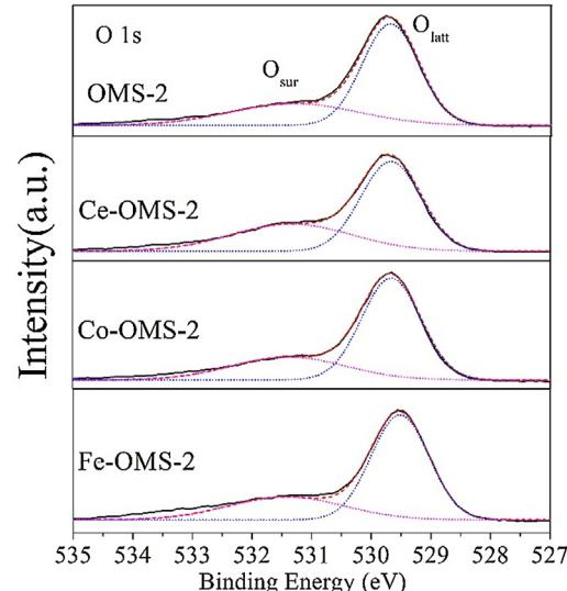
Fig. 9. O1s XPS spectra of OMS-2 and M-OMS-2.
