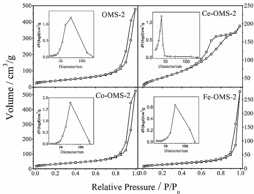
**Fig. 5.**  $\text{N}_2$  adsorption/desorption isotherm for OMS-2 and M-OMS-2 at 77 K. The insert shows the pore size distribution plot calculated by the BJH method.
