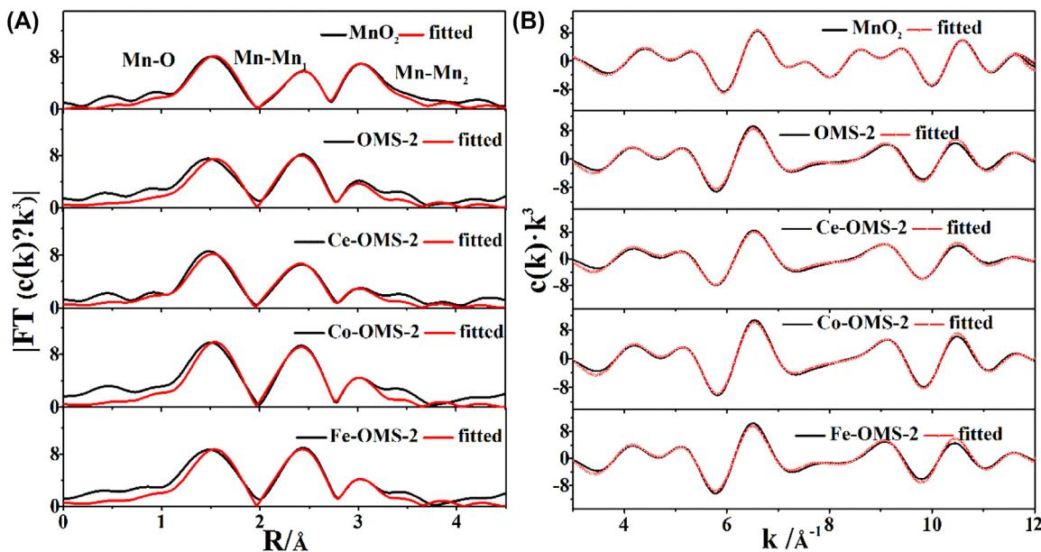
**Fig. 8.** EXAFS spectra of Mn K-edge in series of MnO<sub>x</sub> catalysts: (A) Fourier transforms of filtered  $k^3 \cdot \chi(k)$  into R space, where the red dashed lines correspond to the curve-fitting results; (B) filtered  $k^3 \cdot \chi(k)$  in the k range of 3–12 Å<sup>-1</sup>, where the red dotted lines correspond to the curve-fitting results. (For interpretation of the references to color in this figure legend, the reader is referred to the web version of this article.)
