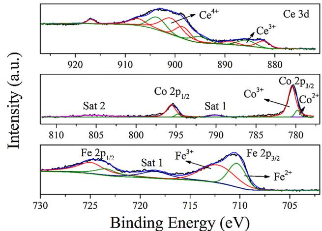
**Fig. 4.** XPS deconvolution spectra of Ce 3d peak of Ce-OMS-2, Co 2p peak of Co-OMS-2 and Fe 2p peak of Fe-OMS-2.
