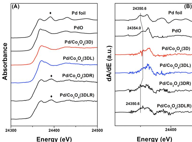
Fig. 8. (A) Normalized XANES and (B) first-order derivatives of XANES of the Pd K-edge in Pd-containing samples and reference samples.
