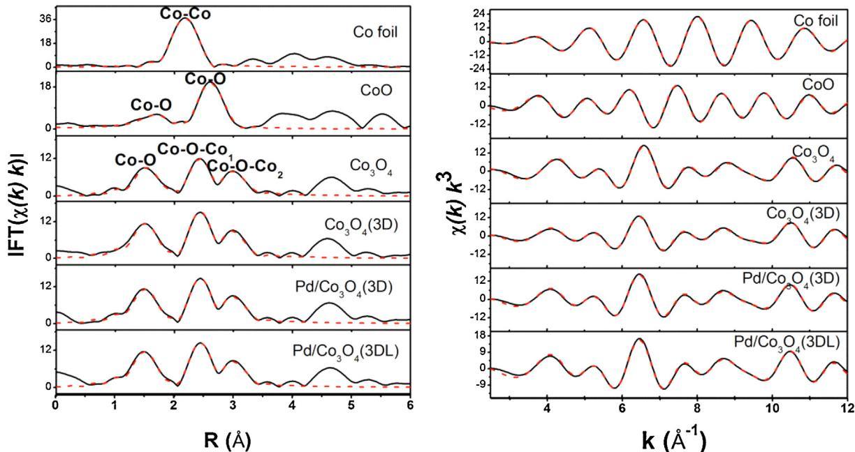
**Fig. 11.** EXAFS spectra of Co K-edge in Co-containing samples: (A) Fourier transforms of filtered  $k^3 \cdot \chi(k)$  into R space, where the dashed lines correspond to the curve fitting results; (B) filtered  $k^3 \cdot \chi(k)$  in the k range of 2.5–13.0 Å<sup>-1</sup>, where the dotted lines correspond to the curve fitting results.
