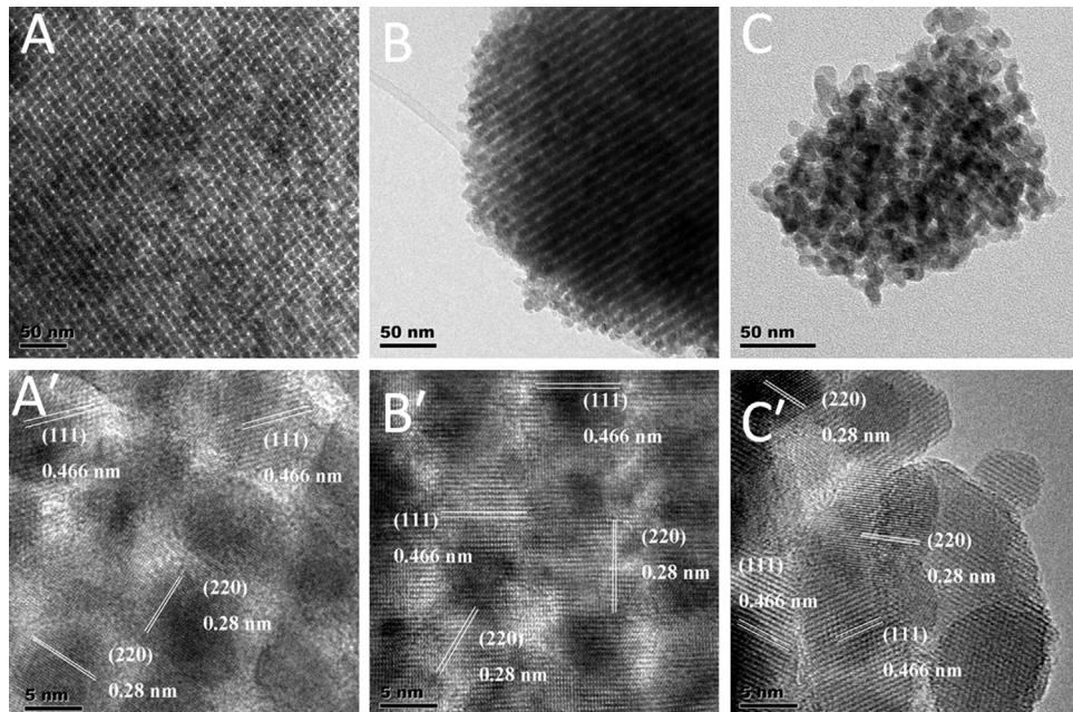
**Fig. 5.** TEM and HRTEM images of the catalysts: (A and A')  $\text{Co}_3\text{O}_4(3\text{D})$ , (B and B')  $\text{Pd}/\text{Co}_3\text{O}_4(3\text{D})$  and (C and C')  $\text{Pd}/\text{Co}_3\text{O}_4(3\text{DL})$ .
