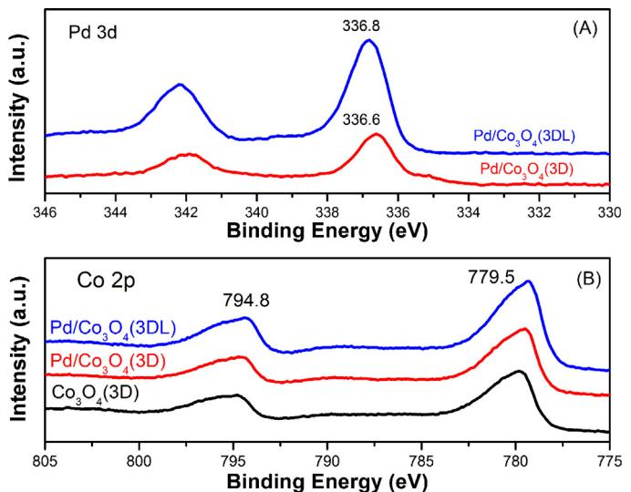
Fig. 7. (A and B) Pd 3d and Co 2p XPS spectra of the Pd based catalysts.
