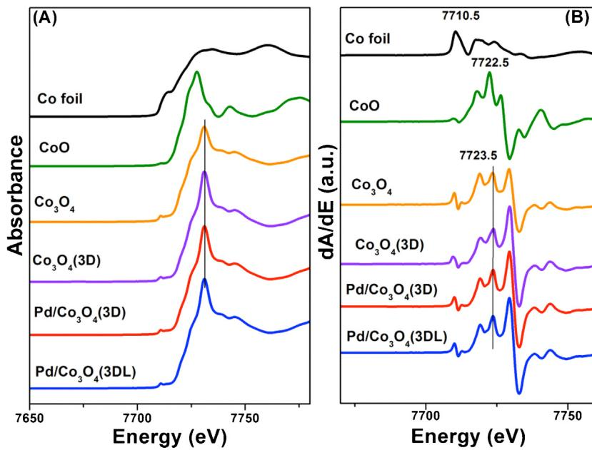
**Fig. 10.** (A) Normalized XANES and (B) first-order derivatives of XANES of Co K-edge in Co-containing samples and reference samples.
