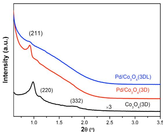
Fig. 2. Low angle XRD of the mesoporous catalysts.
