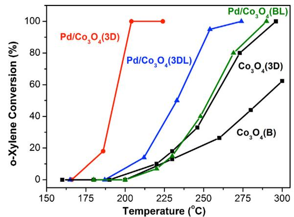
**Fig. 1.** o-Xylene conversion as a function of reaction temperature over the catalysts under the condition of o-xylene concentration = 150 ppm in air, the total flow is 100 mL min<sup>-1</sup>.
