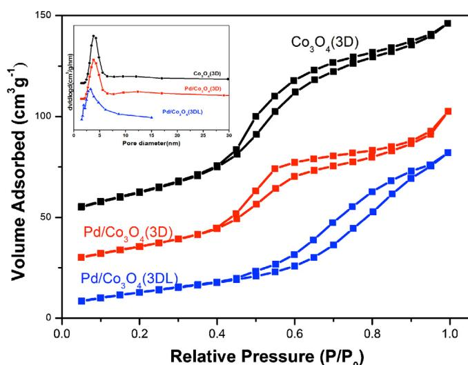
Fig. 4.  $\text{N}_2$  adsorption–desorption isotherms and pore size distributions of the catalysts.
