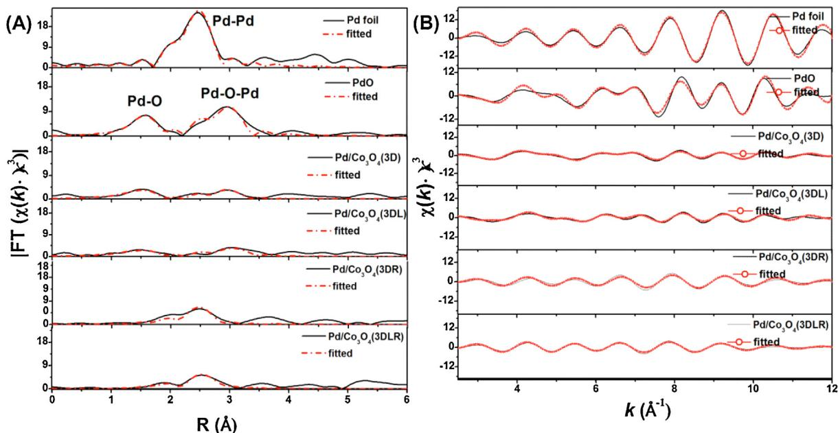
**Fig. 9.** EXAFS spectra of Pd K-edge in Pd-containing samples and reference samples: (A) Fourier transforms of filtered  $k^3 \cdot \chi(k)$  into  $R$  space, where the dashed lines correspond to the curve fitting results; (B) filtered  $k^3 \cdot \chi(k)$  in the  $k$  range of 2.5–12.0  $\text{\AA}^{-1}$ , where the dotted lines correspond to the curve fitting results.
