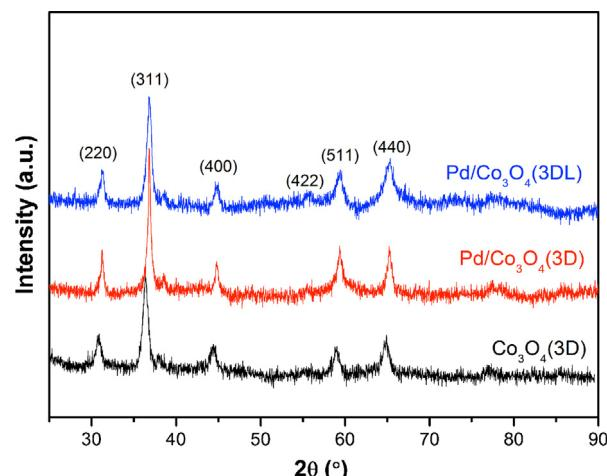
Fig. 3. The large angle XRD of the mesoporous catalysts.
