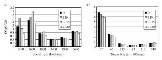
Fig. 6. Comparison of CO emissions, a: full load; b: n = 1900 rpm. D: diesel fuel; B20:20:80 (v/v) blend of methyl soyate: diesel fuel. BE15:12:3:85 (v/v) blend of methyl soyate:ethanol:diesel fuel. BE20:16:4:80 (v/v) blend of methyl soyate:ethanol:diesel fuel.
