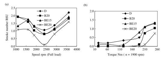
Fig. 2. Comparison of Bosch smoke number for test fuels, a: full load; b: n = 1900 rpm. D: diesel fuel; B20:20:80 (v/v) blend of methyl soyate: diesel fuel. BE15:12:3:85 (v/v) blend of methyl soyate:ethanol:diesel fuel. BE20:16:4:80 (v/v) blend of methyl soyate:ethanol:diesel fuel.
