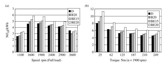
Fig. 4. Comparison of NO<sub>x</sub> emissions for test fuels, a: full load; b: n = 1900 rpm. D: diesel fuel; B20:20:80 (v/v) blend of methyl soyate:diesel fuel. BE15:12:3:85 (v/v) blend of methyl soyate:ethanol:diesel fuel. BE20:16:4:80 (v/v) blend of methyl soyate:ethanol:diesel fuel.
