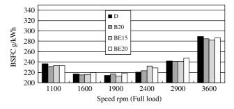
Fig. 1. Comparison of BSFC for test fuels at various engine speeds. D: diesel fuel; B20:20:80 (v/v) blend of methyl soyate:diesel fuel. BE15:12:3:85 (v/v) blend of methyl soyate:ethanol:diesel fuel. BE20:16:4:80 (v/v) blend of methyl soyate:ethanol:diesel fuel.
