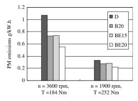
Fig. 3. Comparison of PM emissions for test fuels. D: diesel fuel. B20:20:80 (v/v) blend of methyl soyate:diesel fuel. BE15:12:3:85 (v/v) blend of methyl soyate:ethanol: diesel fuel. BE20:16:4:80 (v/v) blend of methyl soyate:ethanol:diesel fuel.
