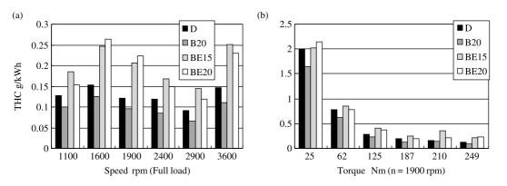
Fig. 5. Comparison of THC emissions, a: full load; b: n = 1900 rpm. D: diesel fuel; B20:20:80 (v/v) blend of methyl soyate:diesel fuel. BE15:12:3:85 (v/v) blend of methyl soyate:ethanol:diesel fuel. BE20:16:4:80 (v/v) blend of methyl soyate:ethanol:diesel fuel.
